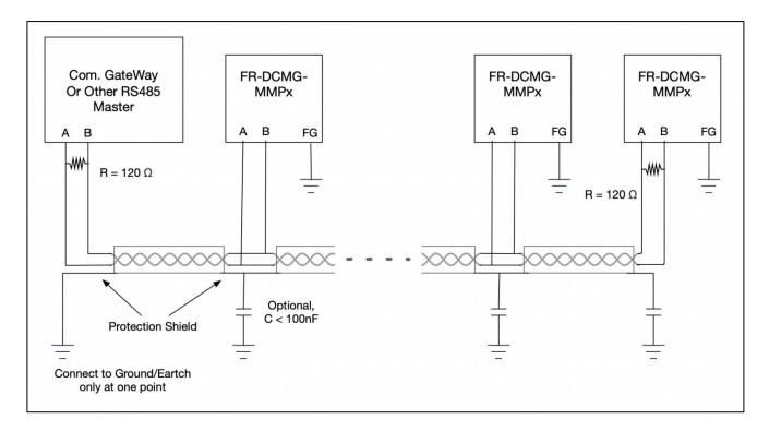
The wiring of on-site communication lines requires that the communication shield can only be grounded at a single point, otherwise there will be a risk of lightning surge damage to all equipment on the entire communication line during a lightning strike;
