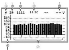
① It indicates that the connected Hall has the arc detection function, and the ordinary Hall does not have this mark;
