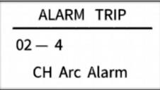
In the figure above: "02" means channel arc fault alarm, and "4" means that the fault arc alarm channel is 4.
